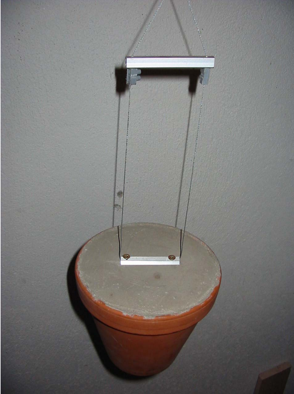
Figure 2 - Fixing the hanging wire to the weight
